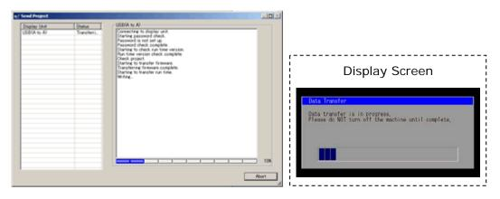
7. When transfer is completed, the status displayed in the dialog box will change from [Transferring] to [Complete Transfer]. Click [Close] to close the dialog box.
