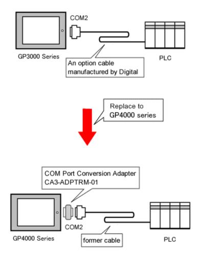
The connection cable for GP/ST-3400 series can be used for GP-4401T.
