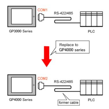
The cable used for connection to GP-3400S via COM2 can be used for GP-4401T only in the following case with a COM Port Conversion Adapter (CA3-ADPCOM-01) added.
