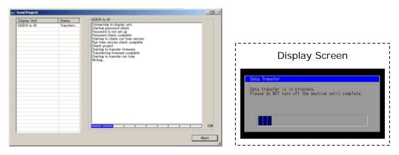
(7) When transfer is completed, the status displayed in the dialog box will change from [Transferring] to [Complete Transfer]. Click [Close] to close the dialog box.
