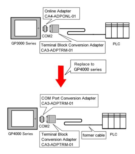
The connection cable for GP/ST-3400 series can be used for GP-4401T.
