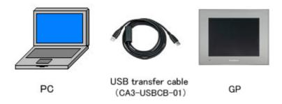
(1) Connect your PC and GP-4501T/TW with a USB transfer cable (model: CA3-USBCB-01).
