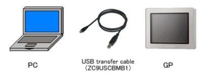
(1) Connect your PC and GP-4301TM with a USB transfer cable (model: ZC9USCBMB1). If the driver of the cable has not been installed on your PC yet, a dialog box will appear. Please follow the instructions.
