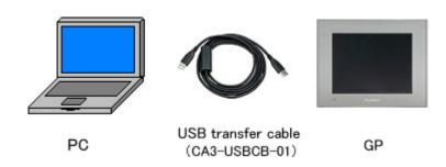
(1) Connect your PC and GP-4501T/TW with a USB transfer cable (model: CA3-USBCB-01). If the driver of the cable has not been installed on you PC yet, a dialog box will appear. Please follow the instructions.
