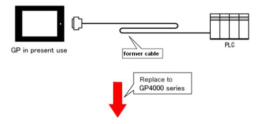
GP-4501T/TW System Configuration (connecting to COM1)
