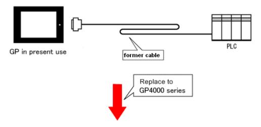
GP-4501T/TW System Configuration (connecting to <a href="COM1">COM1</a>)
