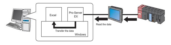
(5) 'Excel' displays the transferred data on the specified cell.
