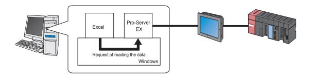
(4) 'Pro-Server EX' reads the Device/PLC data and transfers the read data to 'Excel'.
