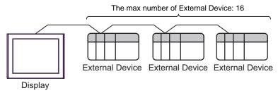
• 1:n connection (For JU series with temperature controller feature)
