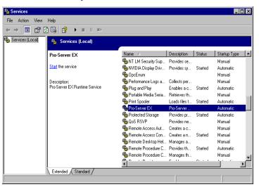
• When you uncheck [Start Pro-Server EX as a service] (normal mode), the "Startup Type" of 'Pro-Server EX' is set to "Manual" on the [Services] screen.
