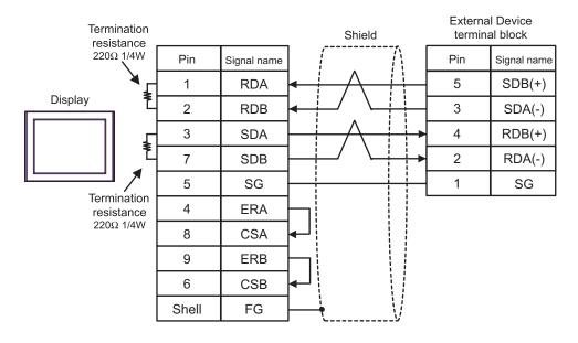
C) Cable diagram using the online adapter (CA4-ADPONL-01), the connector terminal block conversion adapter (CA3-ADPTRM-01) by Pro-face and user-created cable
