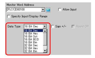
6 Select the [Allow Input] check box to display the [Data Entry] tab. Ensure the [Enable Popup Keypad] check box is selected. You can enter numerical data from the pop-up keypad.
