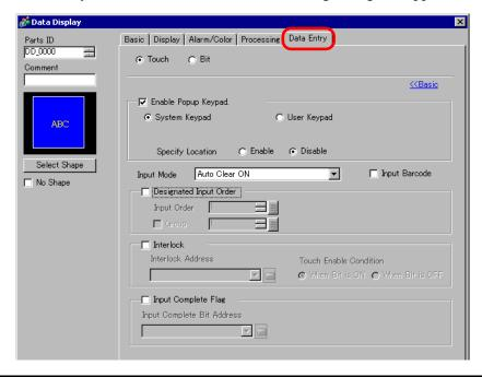
8 Select the [Interlock] check box, then in the [Interlock Address] field specify the bit address (M100) that will enable touch operations.
