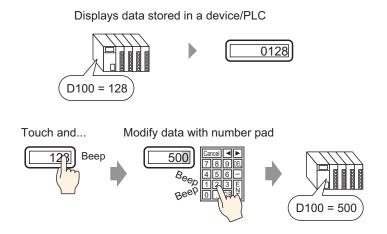
Display data stored in a designated Word Address in the device /PLC as a numeric value. Furthermore, by specifying Input Permission settings, you can display a number pad on the screen and input data to a designated Word Address.
