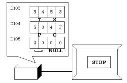
• The relationship of high order and low order Word data will differ according to the device/PLC type.
