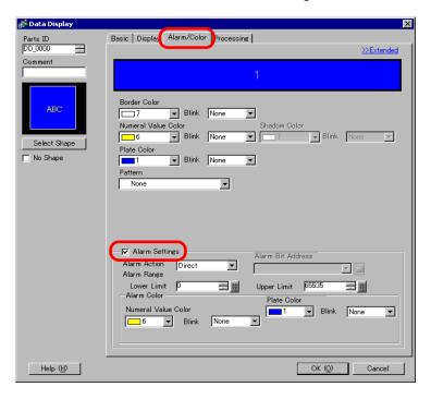
7 In [Alarm Action], select the Upper/Lower Limit Value specification method from [Direct] or [Address] (in this example, [Direct]).
