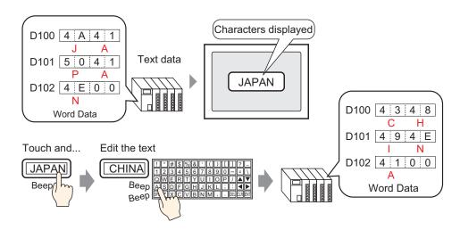
Display text data stored in a specified Word Address on the device (PLC).
