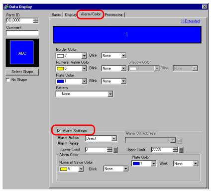
8 In [Alarm Action], select the Upper/Lower Limit Value specification method from [Direct] or [Address] (in this example, [Direct]).
