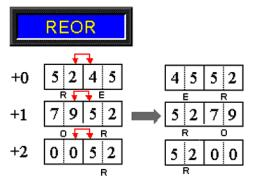
• When you input text to a Data Display set up with integer variables, regardless of how text is set up on the device/PLC, the data displays as follows.
