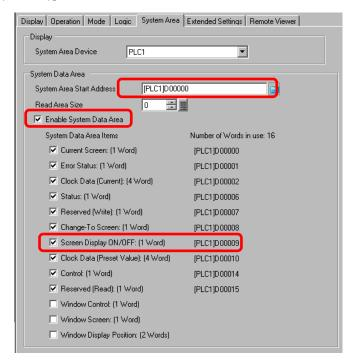
4 Write "FFFFh" to the address displayed in [Screen Display ON/OFF: (1 Word)]. The GP screen display turns OFF.
