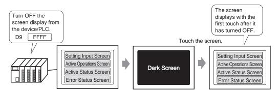
Turns OFF the GP screen display from a device/PLC.
