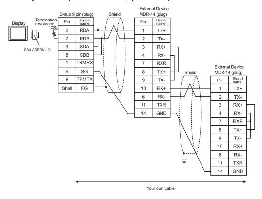
E) When using the COM port conversion adapter (CA3-ADPCOM-01), the terminal block conversion adapter (CA3-ADPTRM-01) by Pro-face and your own cable
