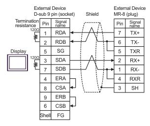
C) When using the online adapter (CA4-ADPONL-01), the terminal block conversion adapter (CA3-ADPTRM-01) by Pro-face and your own cable
