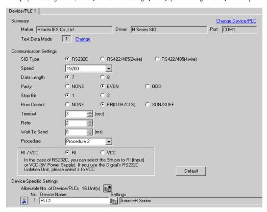
To display the setting screen, click [[Setting]] of the External Device you want to set from [Device-Specific Settings] of [Device/PLC Settings].
