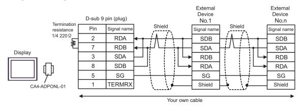
E) When using the COM port conversion adapter (CA3-ADPCOM-01), the terminal block conversion adapter (CA3-ADPTRM-01) by Pro-face and your own cable
