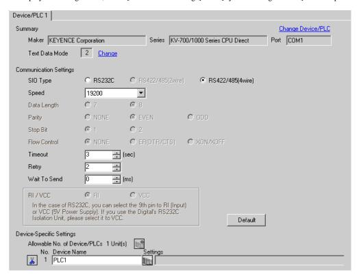
• You can set the speed to 9600-57600 for KV-700 Series, 9600-115200 for KV-1000 Series.
