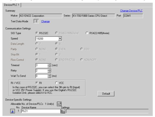
NOTE • You can set the speed to 9600-57600 for KV-700 Series, 9600-115200 for KV-1000 Series.
