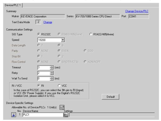
• You can set the speed to 9600-57600 for KV-700 Series, 9600-115200 for KV-1000 Series.
