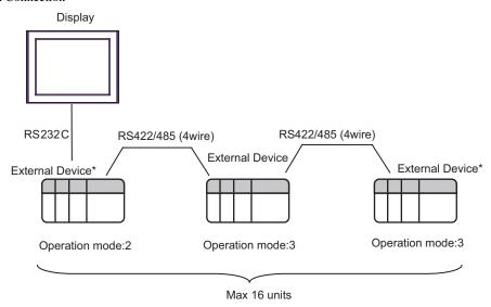
\* Turn ON the termination resistance switch on the interface which terminates the RS422 connection.
