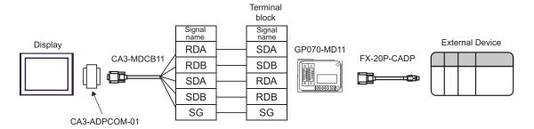
B) When using your own cable, the 2-port adapter II (GP070-MD11) by Pro-face and the connector conversion cable (FX-20P-CADP) by Mitsubishi Electric Corp.
