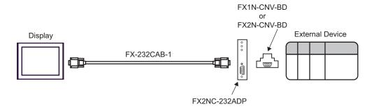
B) When using your own cable, the communication adapter (FX2NC-232ADP) by Mitsubishi Electric Corp. and the function extension board (FX1N-CNV-BD or FX2N- CNV-BD) by Mitsubishi Electric Corp.
