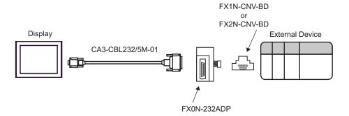
B) When using your own cable, the communication adapter (FX0N-232ADP) by Mitsubishi Electric Corp. and the function extension board (FX1N-CNV-BD or FX2N- CNV-BD) by Mitsubishi Electric Corp.
