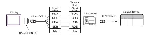
D) When using the online adapter (CA4-ADPONL-01) by Pro-face, your own cable, the 2-port adapter II (GP070-MD11) by Pro-face, and the connector conversion cable (FX-20P-CADP) by Mitsubishi Electric Corp.
