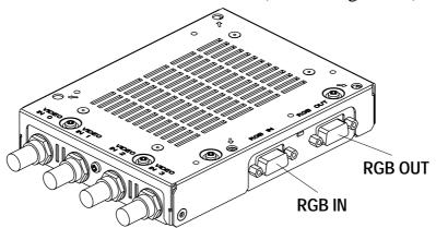
Recommended connector : XM4K-1543 <made by OMRON>
