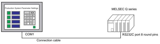
Mitsubishi Q connection cable CA3-CBLQ-01 manufactured by Digital Electronics Corporation (5m) or
