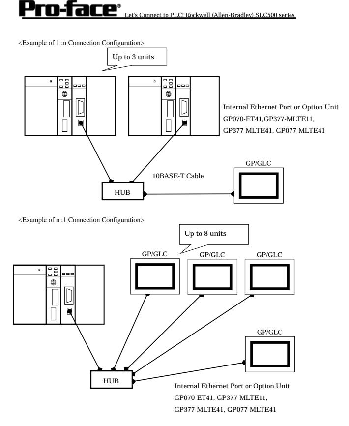
\* There are two types of "full duplex" and "half duplex" for Ethernet communication. Since GP and GLC have half duplex communication, if PLC is a full-duplex type, their communication may be obstructed. Putting HUB in can solve the problem. Use of HUB is recommended.
