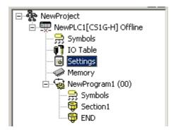
Select the [Peripheral Port] tab on the [PLC Settings] dialog box and set the items as below.
